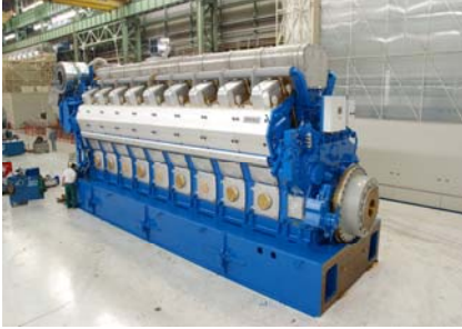
50 bore DF Engine, 950 KW/Cylinder
