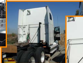
Step 2: Replace with newer truck (Newer truck emits ~35% less NOx and ~80% less PM)
