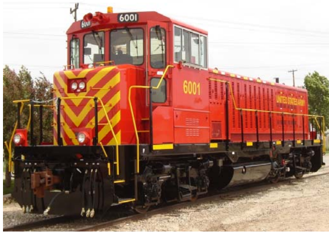
Green Goat™ diesel-battery hybrid switcher, the platform for our fuelcell hybrid locomotives. (Photo courtesy of RailPower Hybrid Technologies)
