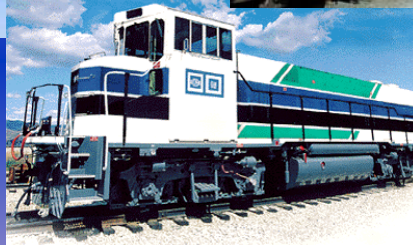
EMD EPA Tier 2 Switch Locomotive
